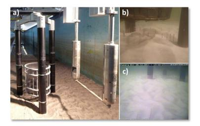
Figure 10 - Tripile-Cage measurements: a) Submergible PIV-Camera device with a passive reflector to detect horizontal level signals in ahead the tripile; b) and c) Investigations on the development of scouring and/or erosion at the pile-mud-zone via imaging recordings with underwater cameras and dip sticks at selected sites (modified after Goseberg et al. 2012; modified after Buck et al. 2012).
