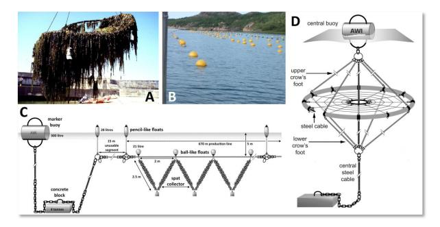
Figure 5 – Aquaculture constructions suitable for the cultivation in high energy environments. (A) Offshore ring design for the cultivation of macroalgae (here: harvesting after grow-out in the harbour of Helgoland), (B) example of a nearshore submerged longline design for mussels and oysters, (C) schematic drawing of a submerged longline suitable for exposed sites, and (D) a technical illustration of the ring design and its mooring system (modified after Buck & Buchholz 2004, Buck 2007).
