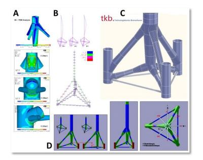
Figure 6 – Modelling of potential attachment points for the combination of longline connections to a tripod foundation. (A) displays alternative connection points, (B) shows the generation of representative loads on the wind energy installation including vibrations, (C) shows the respective tripod foundation for offshore use in depths of about 20-50 meters, and (D) shows the development of a static model (3-5 megawatt class) (modified after Predected 2000)
