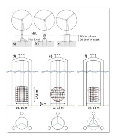
Figure 8 – Lateral view of foundations used for offshore wind energy turbines and different cage designs: a) Tripod; b) Jacket; c) Tripile; d) Cylinder; e) Sphere; and f) triangular prism; MSL = Mean Sea Level. (modified after Schaumann & Dubois 2012; modified after Buck et al. 2012).
